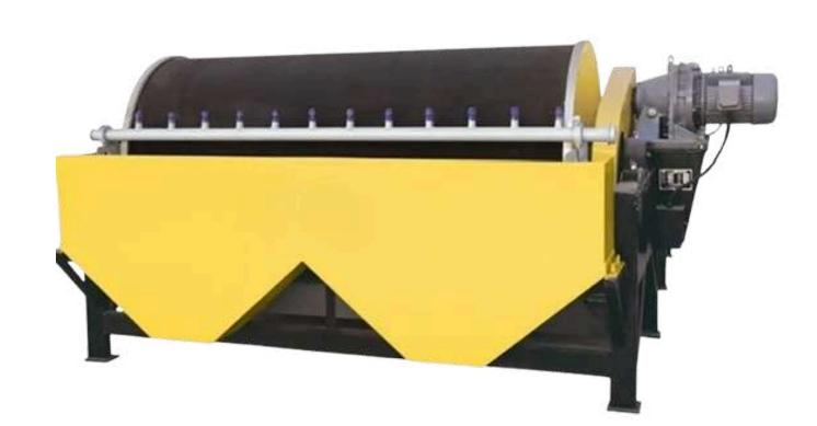
CTB Permanent Magnetic Separator is suitable for processing iron ore and fly ash from iron power plants, offering large capacity and high recovery rates, particularly for selecting iron ore concentrates.
