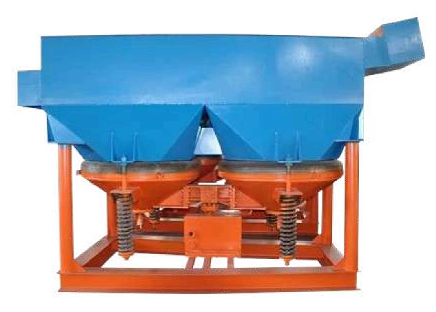
The jig plant (jig machine) belongs to gravity-based equipments, which can separate mineral based on differing of specific gravity. It can be used for separating fine-grained materials as well as coarse materials, with a maximum feed size of 6-8 mm, but in the case of separating alluvial ores in some individual cases, the maximum particle size is 12 mm. Saw-tooth wave jig mainly consists of three parts: main frame, driving set and jigging chamber.
