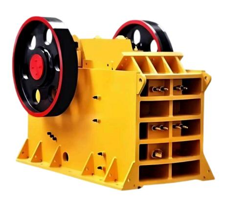
The jaw crusher crushes materials through the periodic movement of the movable jaw. It has high production capacity, a large crushing ratio and high crushing efficiency, and is usually used in the coarse crushing stage.
